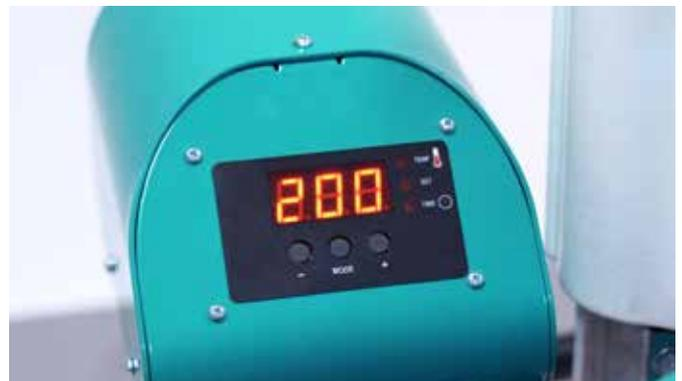
While no LEDs are illuminated, the controller displays the current heater temperature. Press the MODE button to set the TEMPERATURE and TIME.
