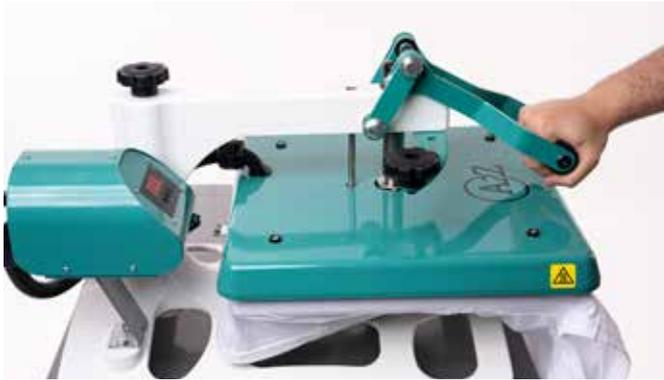
Lower the print handle fully until the upper platen locks into the press position. After the required time has elapsed, lift the print handle.
