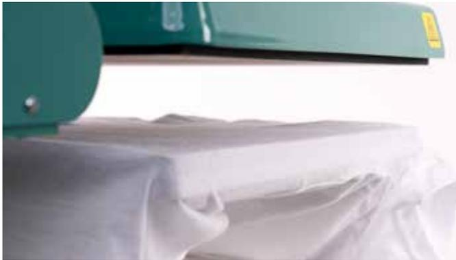
For best results, “thread” the garment around the lower platen so a single layer of fabric is on top of the silicone pad.
