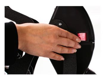
Locate the Power ON/OFF Switch on the side of the press, then turn the Power Switch ON.
