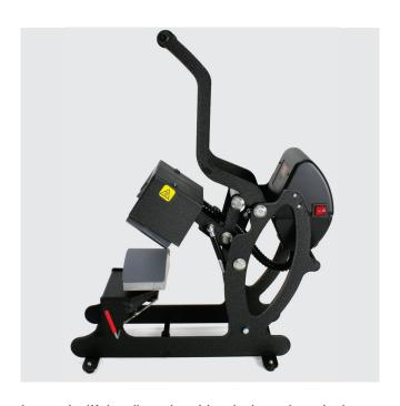
Locate the lift handle and position the heat platen in the UP position.
