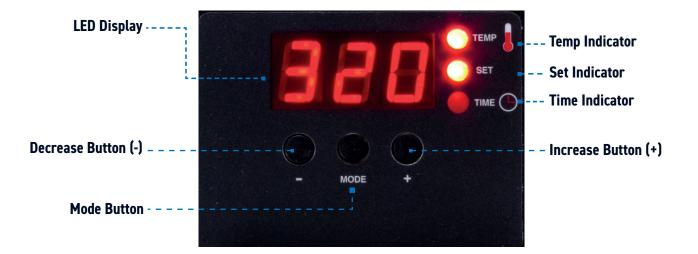
Power: Digital Timer: Digital temperature control: Size of heat platen: Weight: 240 Volt, 500 Watt 1-999 seconds 96-221°C 9 cm x 16 cm approx. 13,5 kg
