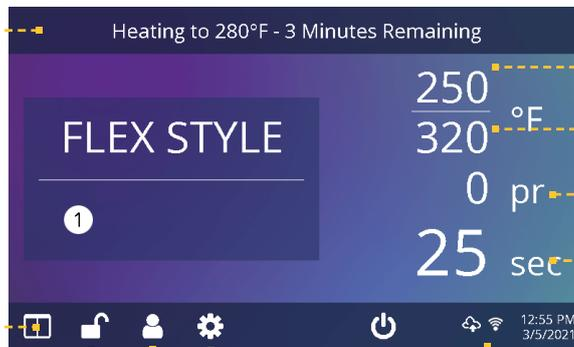
Displays current top heater temperature.
